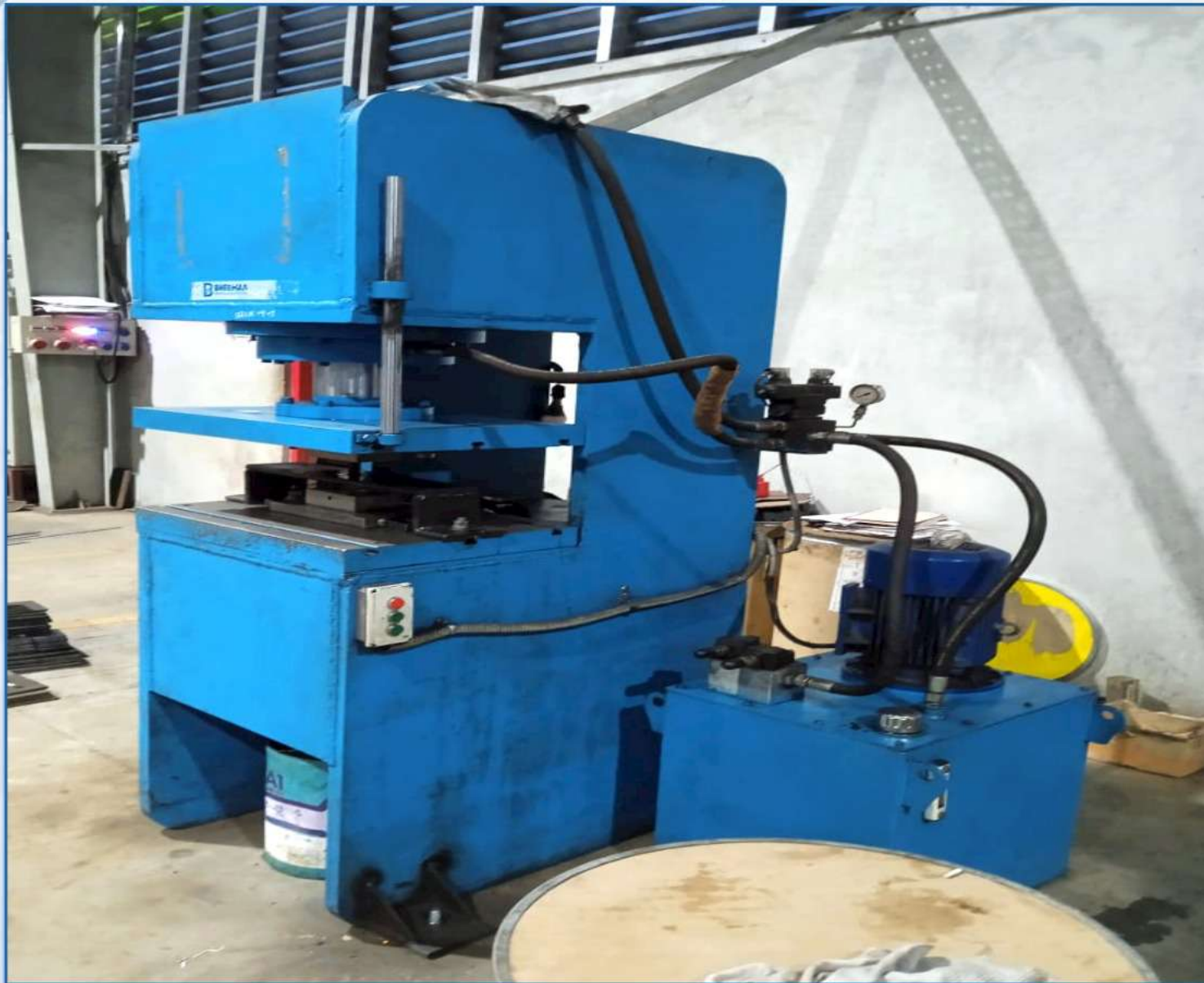
Hydraulic Press Machine: Hydraulic Press Machine of 150 MT capacity for bending purpose.
