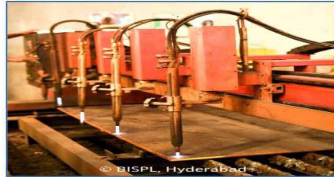
XY - CnC : CNC Shearing Machine capable of cutting sheets up to 100mm thick and supporting lengths of up to 12,000mm.
