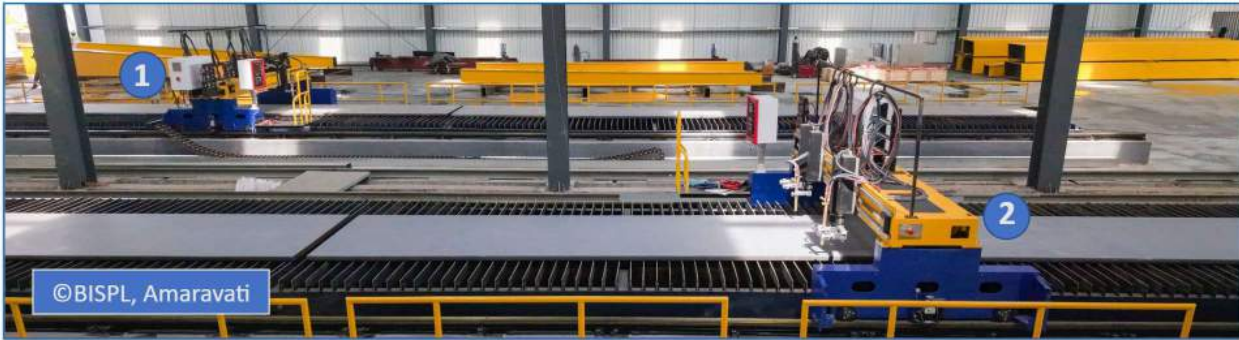
XY - CnC : CNC Shearing Machine capable of cutting sheets up to 110mm thick and supporting lengths of up to 25,000mm.
