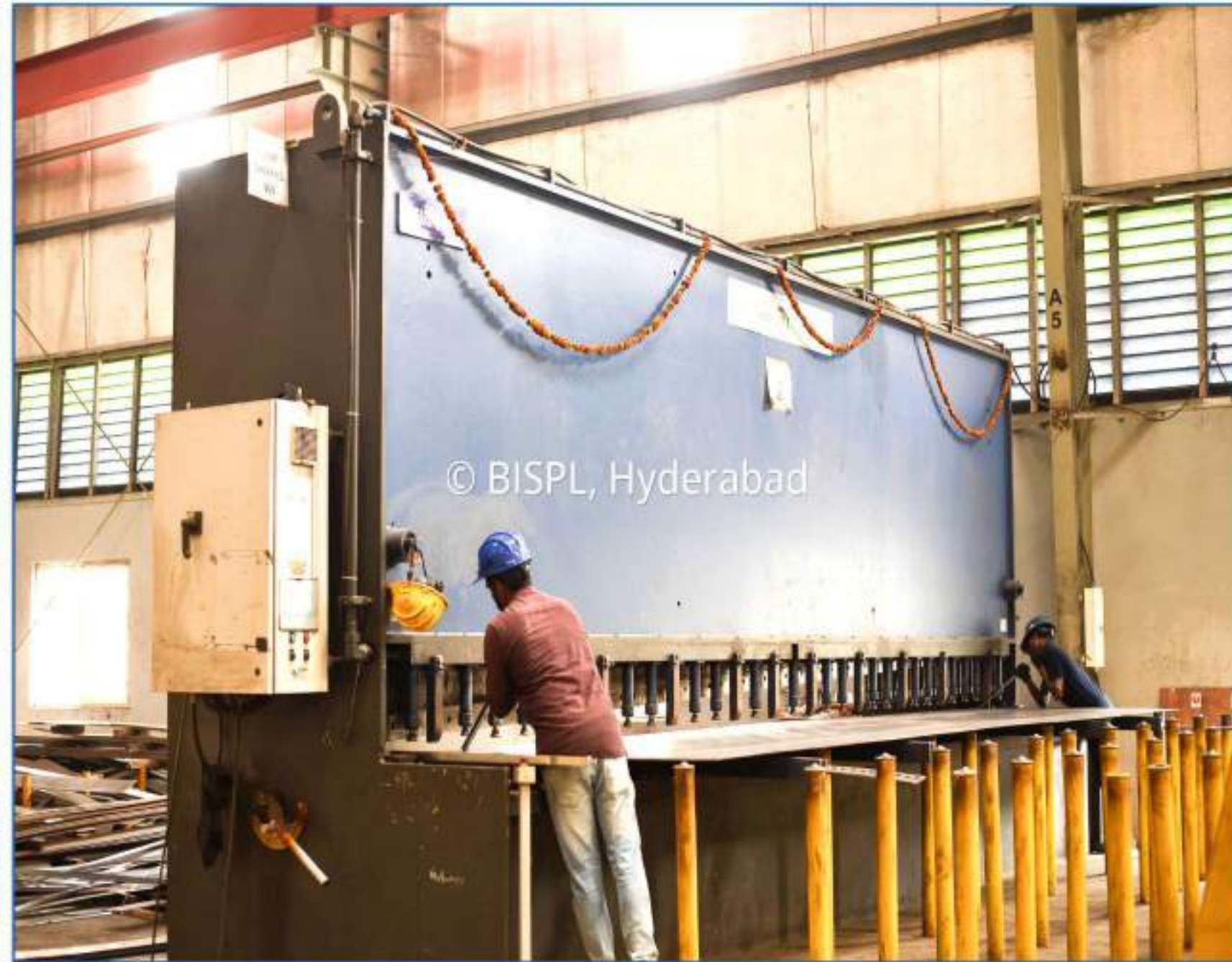
Shearing Machine : With shearing capacity up to 16 mm thick plate. For the length of 6700 mm.
