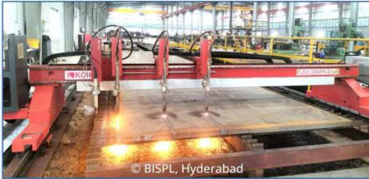
XY - CnC : CNC Shearing Machine capable of cutting sheets up to 100mm thick and supporting lengths of up to 12,000mm.
