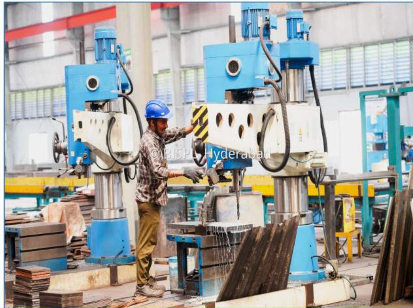
Radial Drilling Machine: Radial Drilling Machines with Boring capacity Up to 85mm .
