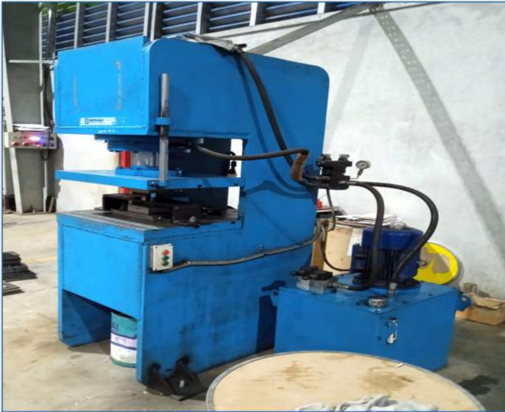
Hydraulic Press Machine: Hydraulic Press Machine of 150 MT capacity for bending purpose.
