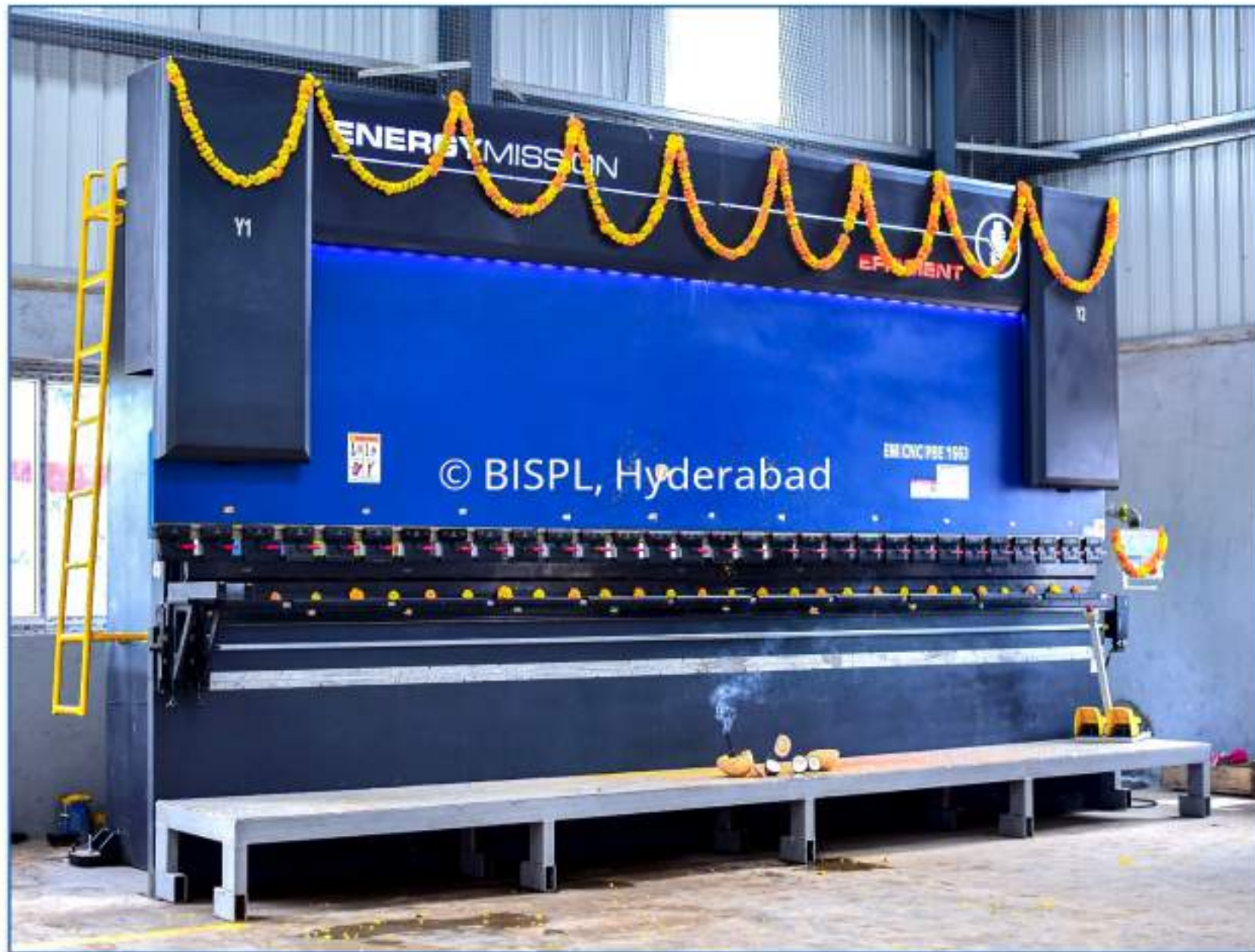
Press Brake: Our Press brake has the bending range of 0.5 – 3 mm thick sheet up to the length of 6300 mm .
