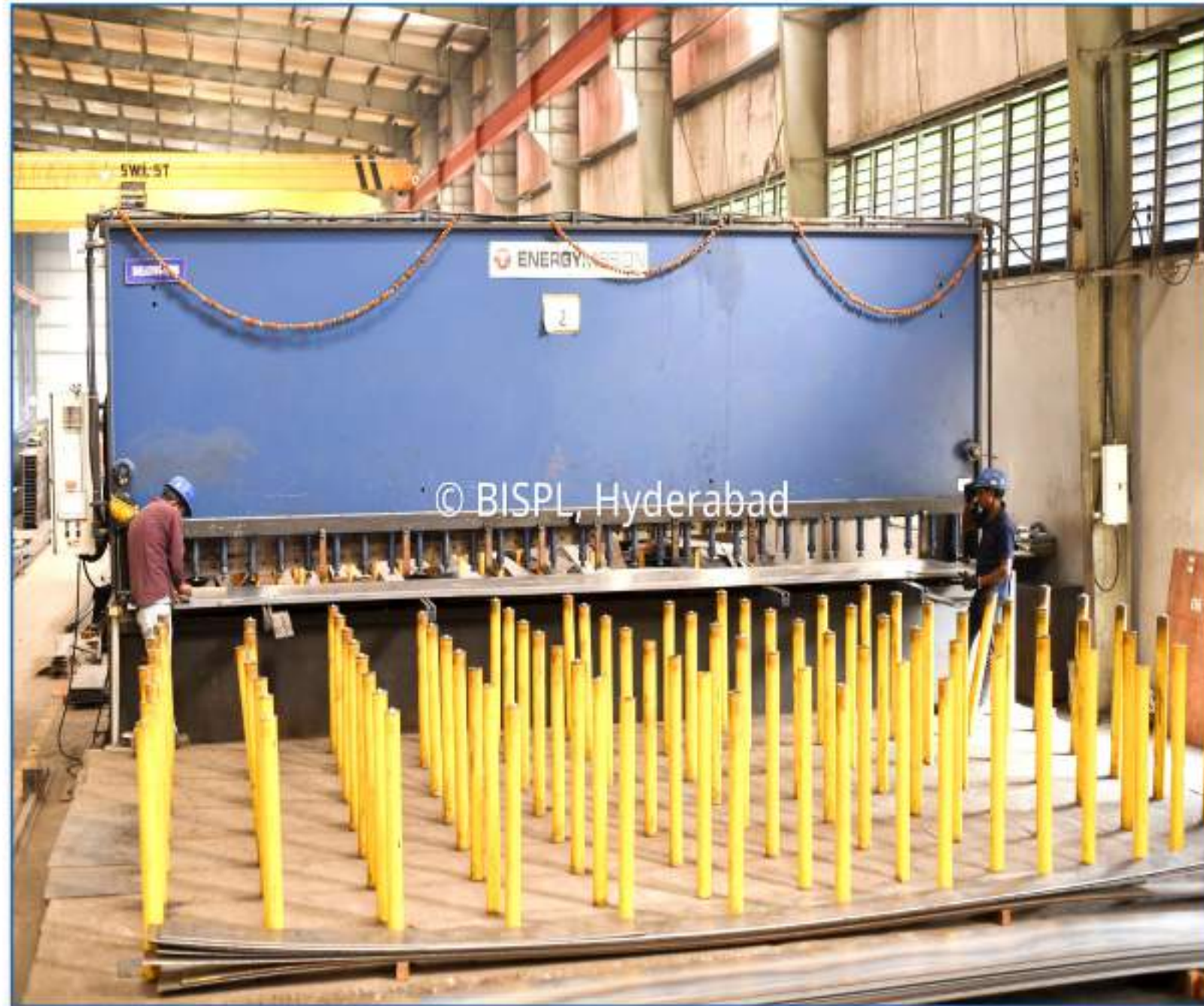
Shearing Machine : With shearing capacity up to 16 mm thick plate. For the length of 6700 mm.
