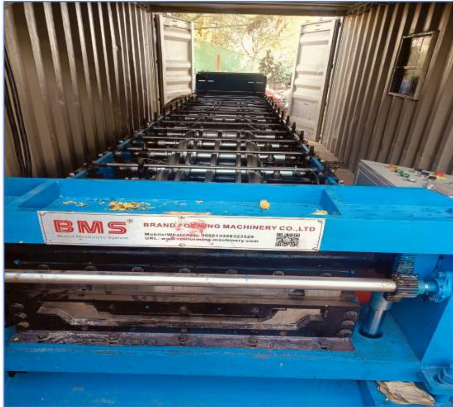
Standing Seaming Machine: It has the capacity of 300 mpa, supports coils with widths of 610/730 mm and handles material with a thickness of 0.5 mm.
