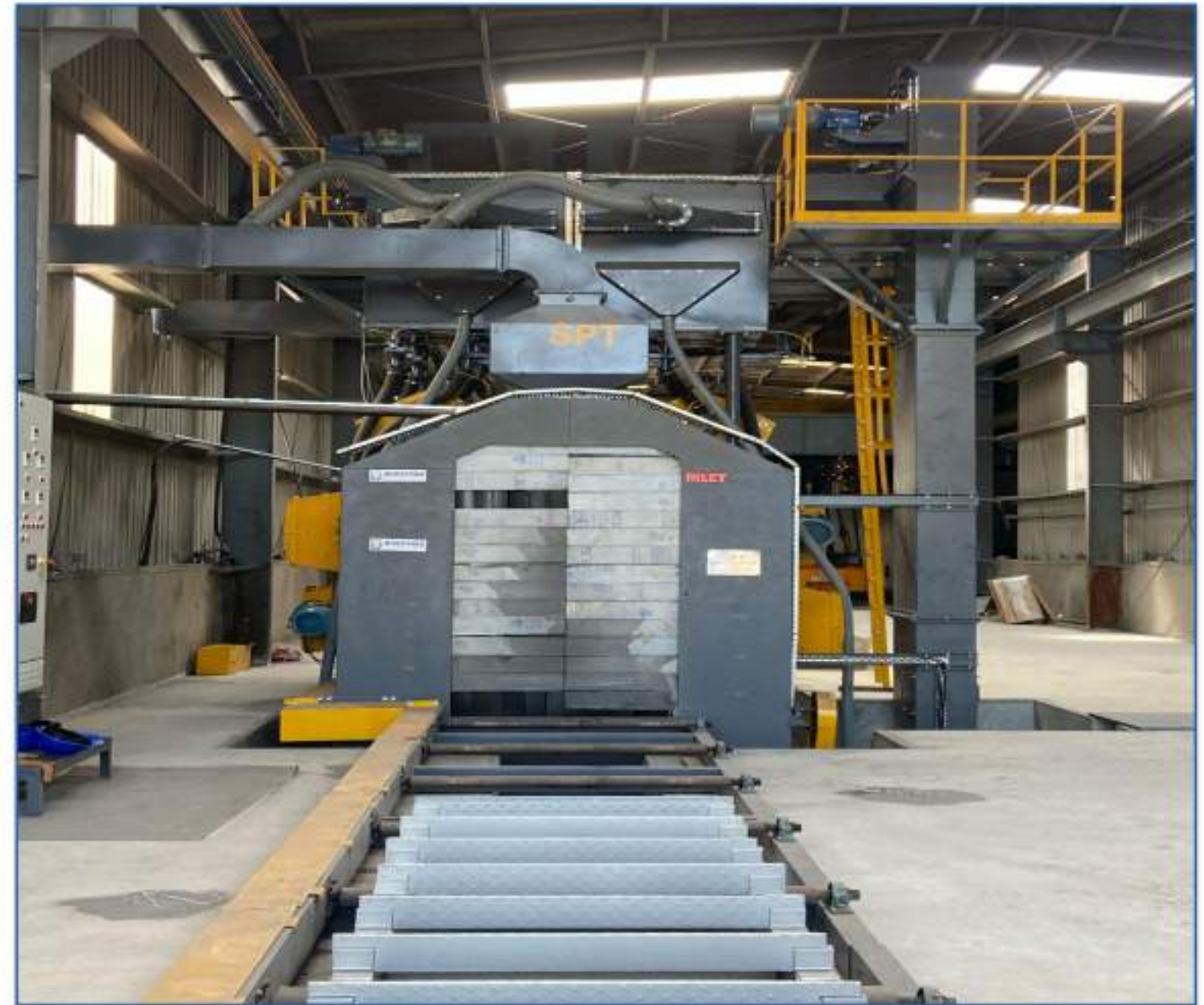
Fully Automatic Shot Blasting - Machine: with an opening of 2.2 meters in height and 1.2 meters in width.
